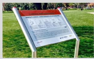
In accordance with the EN 16630:2015 safety standard, a signboard, clearly recognisable as such, is required where outdoor-fitness equipment is installed.
